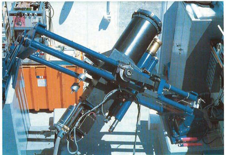
Figure 1: The 36-cm telescope of the H\alpha Survey at La Silla. Assembled and tested on the sky at Marseille Observatory in April 1989, it was installed at La Silla in October 1989. Its shelter, built by ESO, has a sliding roof, and an adjacent room has been added to accommodate the data-acquisition and visualization system. Below the main tube one can see two small refractors: one is equipped with a small CCD camera for guiding and the other one with a normal eyepiece for field identification. Prominent at the lower part of the instrument are the bright cryostat containing liquid nitrogen for cooling the photocathode of the Photon-Counting Camera (dry nitrogen circulates inside the pipes to prevent frost formation on the photocathode) and the High-Voltage power supply (black box).
