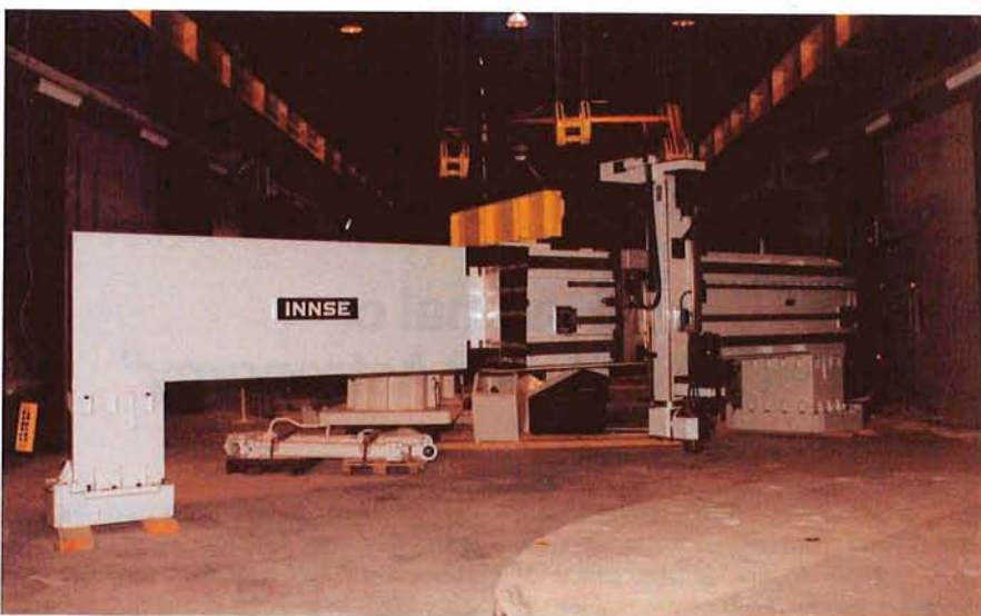
Figure 3: Milling bridge. This bridge, which has a free span of 9 metres, will be installed over the grinding machine rotating table. The picture shows the computer-controlled carriage which bears the milling head.
