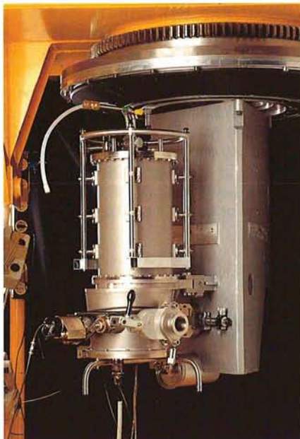
Figure 1: IRAC 2 mounted on the telescope simulator during testing in Garching.
