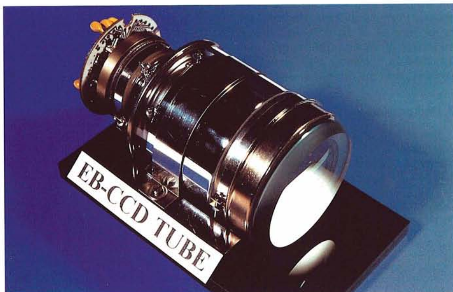
Figure 1: Tube assembly of the electron-bombarded CCD built by LEP.
