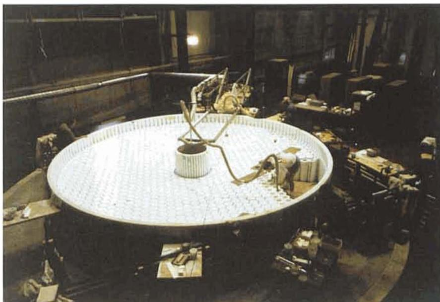
Figure 3: Preparation for fabricating the first 6.5-m borosilicate honeycomb mirror. The 6.5-m mould under construction. At the time of the Conference, the 6.5-m mirror had already been cast.
