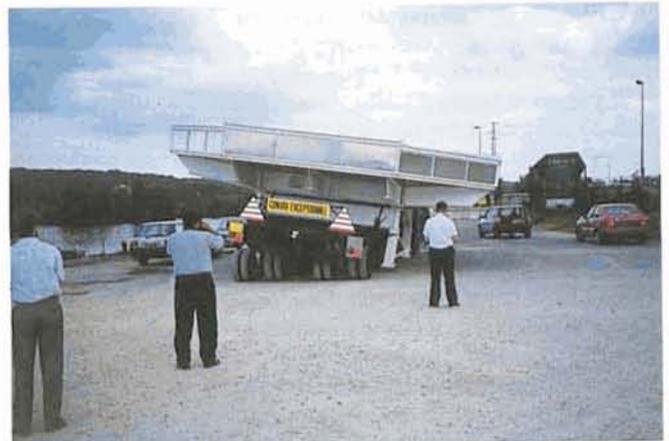
Figure 3: "Rock-and-roll" test on the hydraulic platform.
