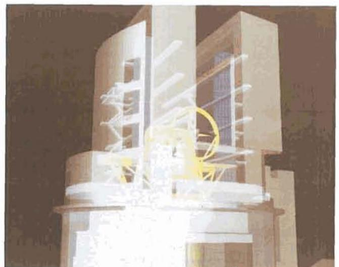
Figure 7: The Japan National Large Telescope Project (diameter of the primary: 8.3 m). Enclosure concept: there are two large walls ("great walls"), one on either side of the telescope in order to channel and flush the air flow. Front, back, and side ventilators are provided. The enclosure will be air conditioned in the day time (from K. Kodaira, National Astronomical Observatory).
