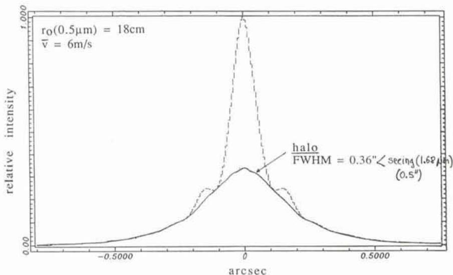
Figure 9: Experimental PSF at  $1.68 \mu$  obtained with the COME-ON system with a seeing of  $0''.5$  with the ESO 3.6-m telescope. The image is composed of a halo (continuous line) of  $0''.36$  FWHM and a sharp core (broken line) which has the width of the Airy pattern of the telescope (F. Rigaut, G. Rousset et al. COME-ON experiment).
