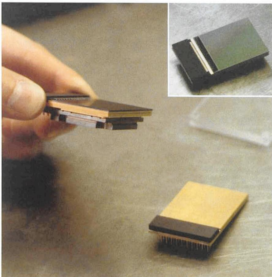
Figure 1: The first-front side sample of the described Thomson 2048<sup>2</sup> CCD during inspection at ESO (left), together with a "package sample", i.e. the support without the chip (lower right). A view of the sample almost face-on is shown in the insert.
