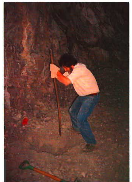
Figure 7: Obtaining accurate microseismic measurements free from external disturbance such as wind buffeting requires the seismometer to be buried on firm rock at least 40 cm below the surface, and requires a polyvalent seismologist! Here, Luis Rivera is at work in the excavation of telescope No. 4.
