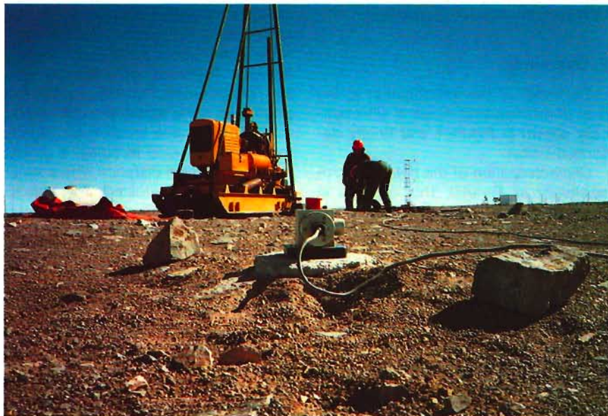
Figure 4: View of the geophone (foreground) and of the hammer-handling machine (background) used to measure the GVTF.
