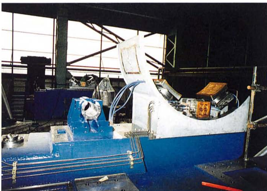
Figure 3: Altitude hydrostatic bearing pads and locking pin support.
