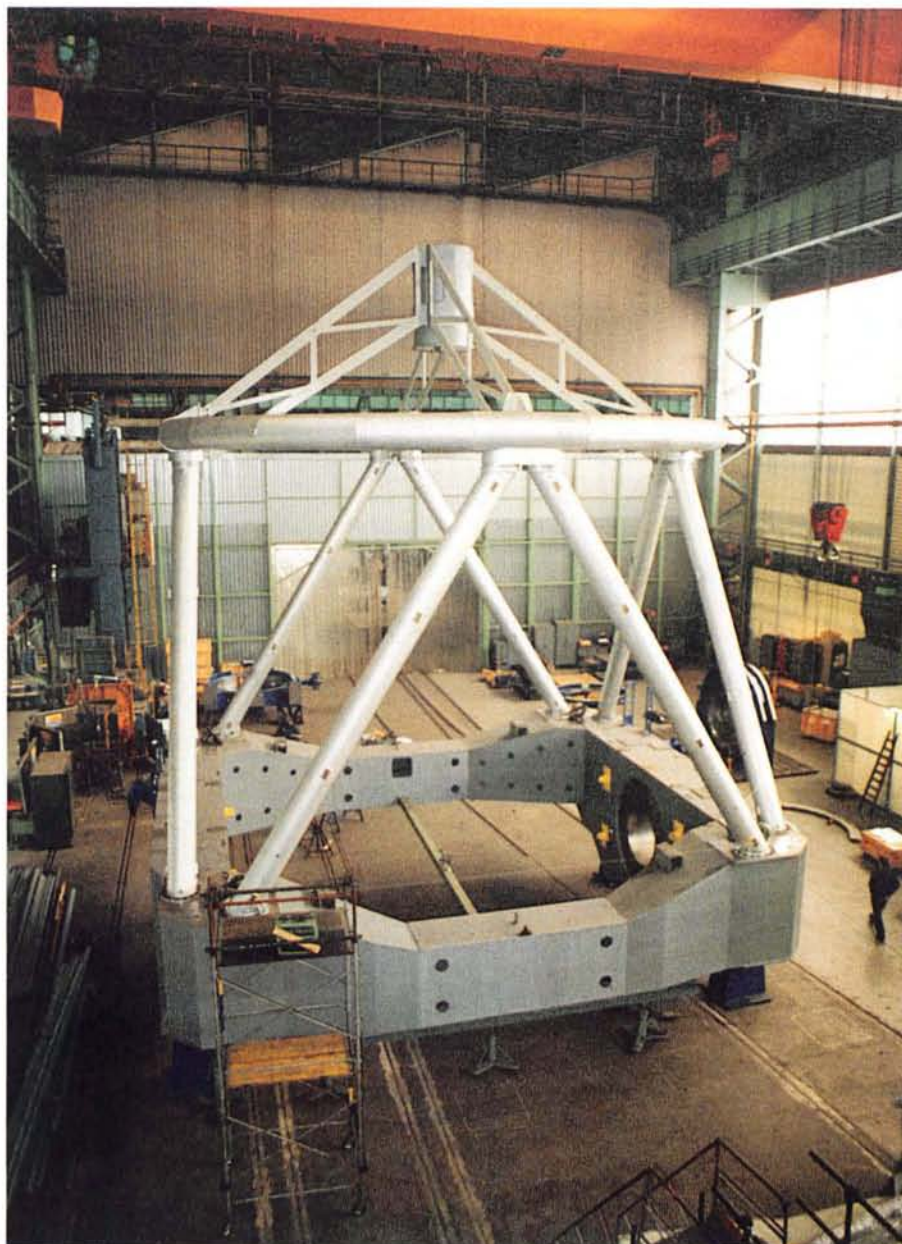
Figure 2: The tube is placed on supports for the Top Unit dynamic test.
