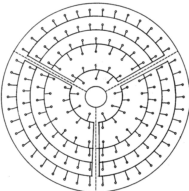
Figure 3a: Topology of axial support hydraulic circuits.
