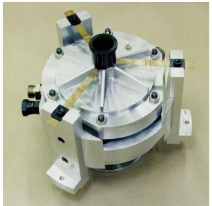
Figure 3b: Passive axial support prototype.
