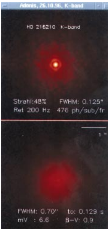
Figure 1: Adonis K-band 10-sec-exposure image of a point source obtained at the 3.6-m telescope on La Silla (top). The look-up table is power 1/4th in order to highlight the low level features. The corresponding uncorrected 10-sec-exposure image is shown at the bottom.
