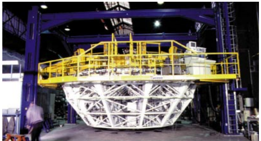
Figure 4: The M1 cell and M1 dummy is lifted by the handling tool.
