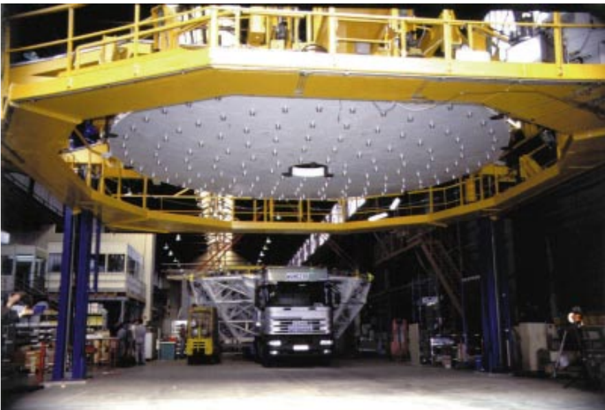
Figure 3: The M1 cell is brought below the M1 dummy hanging in the handling tool to test the integration procedure.
