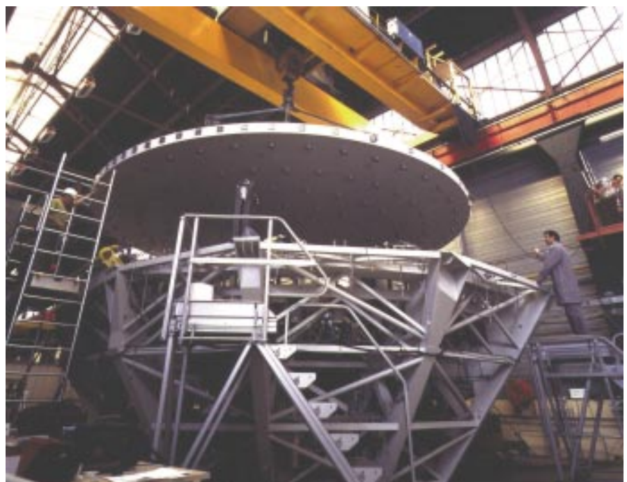
Figure 1: First integration of the M1 dummy mirror in the cell.
