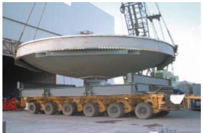
Figure 2: The VLT coating plant in front of the Mirror Maintenance Building on Paranal. After removal of the upper part of the vacuum chamber, the lower part is lifted off the carriage, allowing a good view of the individual parts, including the rigid transport structure. ▼
