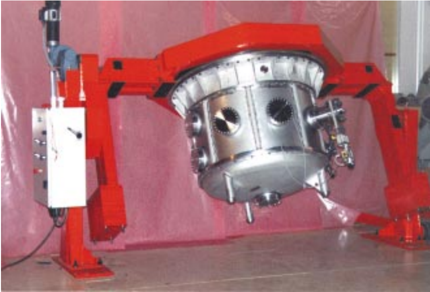
Figure 3: Test equipments of VISIR. One can see the test cryostat mounted on its integration support, which allows to simulate the telescope position and to measure the mechanical flexure.
