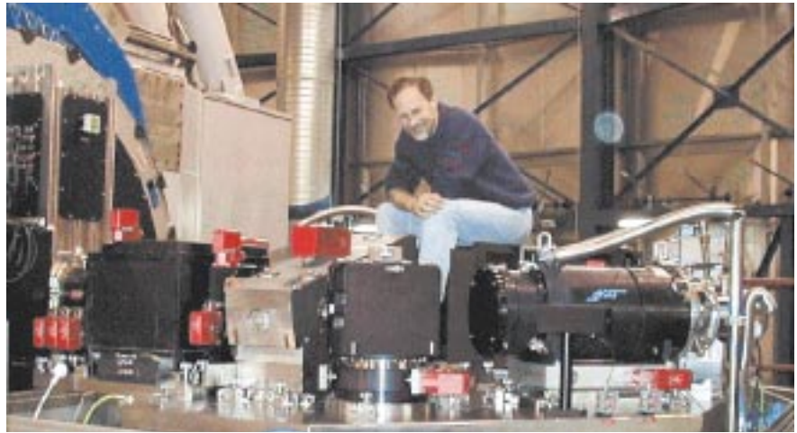
Figure 2: During the frantic days of the instrument integration at the telescope, J.L. Lizon takes advantage of the robust design of the UVES functions for a short rest. Most of the sub-systems are already mounted on the table fixed to the Nasmyth platform: from the left the preslit units, the shiny back of the blue echelle mount, the blue CD unit, camera and CCD.
