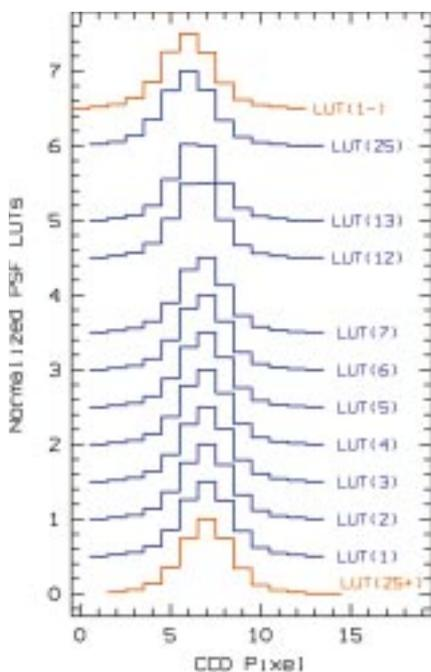
Figure 1: Attempt to represent the Look-Up-Table (LUT) used for the prediction of the Spectral PSF (SPSF) at any wavelength bin of the 2D spectrum. In this example, the increase in sampling ( $n$ ) is 25 and the length of the SPSF ( $l$ ) is 13. Each LUT entry (a row in Fig. 1) is a string of 13 numbers making up a single SPSF realisation (see Section 2).
