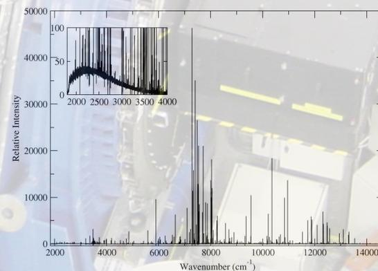
Figure 1: Overview spectrum of a Th-Ar lamp. Wavelength range is 715 nm to 5000 nm ( $14000 \text{ cm}^{-1}$  to  $2000 \text{ cm}^{-1}$ ). The line intensity is given in arbitrary units. The inset shows that longwards of  $2500 \text{ nm}$  ( $<4000 \text{ cm}^{-1}$ ), thermal emission from the hot cathode produces a continuum that underlies the pure emission line spectrum.
