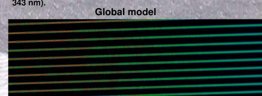
Same plot as to the left, except that the Gaussian centroid and width are fitted using two-dimensional (3, 3)-degree polynomials as function of wavelength and order number (only  $4 * 4 + 4 * 4 = 32$  free parameters). This exploits the fact that the spatial profile is expected to vary slowly as function of wavelength and from one order to the next, and allows interpolating the regions with no signal, leading to a regular (better) object tracing.
