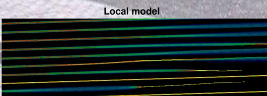
Reconstructed order traces using an order-by-order model where each of the 33 orders (only 10 orders shown) is modelled by a Gaussian whose centroid and width vary as 3rd degree polynomials. The irregular shape of the traces indicates that the large number  $((4 + 4) * 33 = 264)$  of free parameters cannot be reliably determined from the low S/N quasar data.
