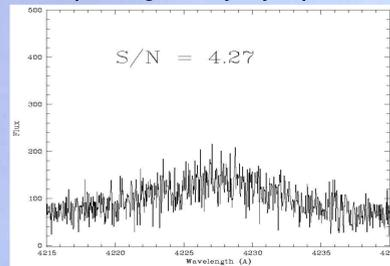
The spectrum signal-to-noise (S/N) may be improved by summing only the few (in this example 4) pixels at the slit center, which contain most of the object signal. Problem: The object flux outside the extraction window is lost.
