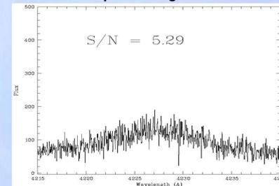
Horne showed that the optimal S/N is achieved using a weighted sum of all pixels, with weights proportional to  $p/V$ , where  $p$  is the relative illumination fraction (spatial profile), and  $V$  is the pixel flux variance.
