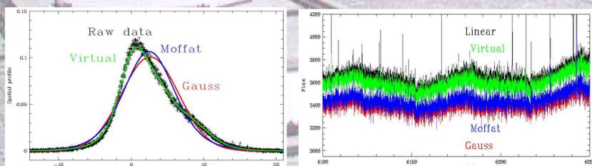
The object spatial profile (black), two analytical (Moffat/Gauss) models and the non-analytical Virtual model. Clearly, the asymmetrical object spatial profile is well fitted only by the non-analytical model. (The high asymmetry in this data is due to an asymmetric source and is not representative of the UVES spatial profile for a point source.)
