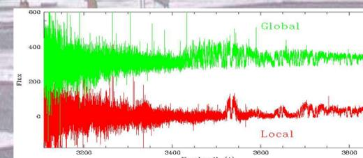
Extracted spectra from the global/local models described below (the global spectrum is shifted +300 units for easier comparison). The local model fails to properly trace some of the orders, which causes spuriously low flux in parts of the Lyman-alpha forest (> 343 nm).
