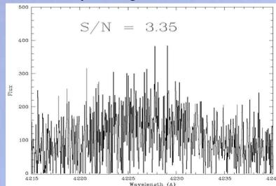
The straightforward way to extract the data is to sum all pixels along the slit, for each wavelength. Problem: Pixels near the slit edges contain little or no signal, but contribute with noise, leading to a noisy spectrum (simulated data).
