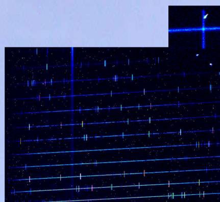
Raw UVES image (and a zoom) showing 12 echelle orders, sky emission lines (vertical) extending over the entire slit and cosmic ray hits (white dots). The data reduction is simplified by the fact that the cross-dispersion direction is aligned with the detector columns (QSO-1101-264).
