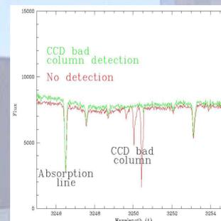
Extracted spectrum showing the effect of detecting and handling CCD defects. Kappa-sigma clipping is used to detect outlier pixels, which are then excluded from the optimal extraction. The three absorption features around 325 nm are due to the CCD defect and might be mistaken for real absorption lines, if not handled. Also note that the very weak absorption feature at the beginning of the CCD defect is recovered.
