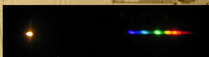
*"Looking through the spectroscope at a fluorescent lamp... one violet line at 4360Å and one green line at 5460Å. If the lines are not exactly in place, the difference must be added or subtracted respectively in all determinations"*
