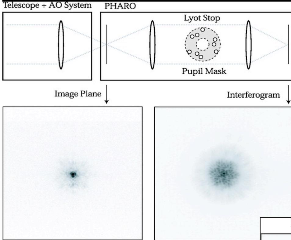
Placing an aperture mask in the pupil plane allows calibration of atmospheric turbulence on scales larger than the subapertures. Coupled with AO (for overall wavefront stabilization), it filters almost all noise from turbulence and AO errors. This yields very stable performance.
